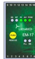
LIFT STOPPED WITH OPEN DOORS
